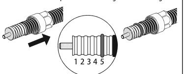
Push the collet back over the O-ring until it stops, then release it. Verify that the collet has located into the first corrugation. DO NOT TWIST. Clean off face of foam with alcohol wipe.
