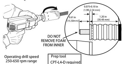
If all of the outer jacketing wasn't removed during initial cable prep remove at this time. Slide the clamping nut over the cable end. Install pre-lubricated o-ring in the 5th corrugation.
