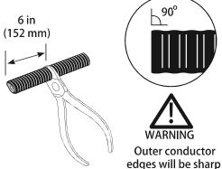
Apply forward pressure until you feel the ball bearings land in a corrugation valley. Reverse tool to remove. End of the prep tool can be used as a guide.
