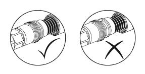
9 Slide the clamping nut up to the outer body and tighten by hand by turning the clamping nut and holding the front body stationary. Complete the installation by tightening with torque and open ended wrenches.
