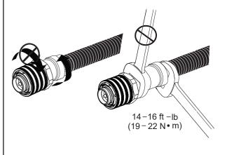
Slide the outer body over the collet and rotate slightly to align socket within the outer body with the hex edge on the collet. Push until fully engaged.
