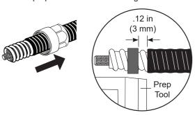
Apply a thin layer of grease to the gasket. Slide the collet over the gasket until it stops, then thread onto the corrugations and use a 16 mm wrench on the collet flats rotating until 2.4 mm of outer extends past the face of the collet. Pull outer body to remove coring bit from the tool and use guide mark to verify outer length.
