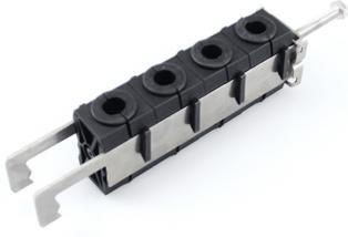
KwikClamp™ Hanger for power & fiber cables, 4.5-9 mm, quadruple stack, round or flat mounting; includes hardware
