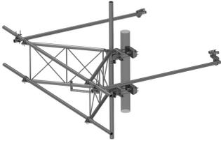
G23RHDXL PIM OPTIMIZED SPACING High Capacity Sector Frame with extended 10' Spine for RRU Mounting & extended frame for sites requiring increased sector to sector antenna spacing. 2 7/8in OD x 12.5ft face. Antenna pipes sold separately.
