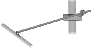
Large Leg Tieback Bracket / Stiff Arm, 2-3/8" OD x 10 ft Pipe with Attachment Hardware, for up to 16" OD or 60 degree angle tower leg
