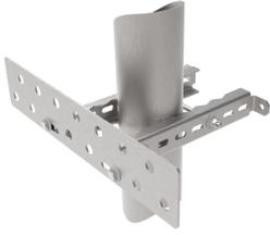
PIM-Guard® Antenna and RRU Cable Support Bracket with 13 ports for stackable hangers (up to 3 per port). Install with torque wrench set at 10 to 15 ft-lb to meet carrier PIM requirements.
