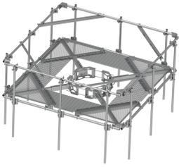
Four-sector HD Platform for 10" to 30" Monopoles, 12ft x 3.5" OD Face pipes, 2.88" OD Top Rail, includes (12) 2.88" OD x 96" antenna pipes
