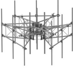
G23RHDXL PIM OPTIMIZED SPACING High Capacity Monopole platform with extended 10' Spine for RRU Mounting & extended frame for sites requiring increased sector to sector antenna spacing. 2 7/8in OD x 11ft face with (9) 2-7/8in OD x 96in Antenna pipes
