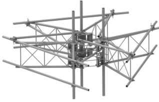
G23RHDXL PIM OPTIMIZED SPACING High Capacity Monopole platform with extended 10' Spine for RRU Mounting & extended frame for sites requiring increased sector to sector antenna spacing. 2 7/8in OD x 12ft face. Antenna pipes sold separately.
