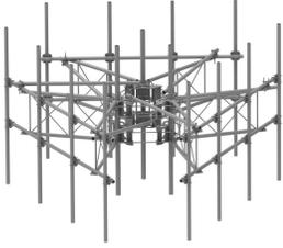
G23RHDXL PIM OPTIMIZED SPACING High Capacity Monopole platform with extended 10' Spine for RRU Mounting & extended frame for sites requiring increased sector to sector antenna spacing. 2 7/8in OD x 13ft face with (12) 2-7/8in OD x 96in Antenna pipes
