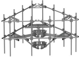
3-Sector Monopole Co-location Platform Kit, 12 in to 50 in OD, 14 ft 6 in face, includes twelve 2-7/8" x 96 in pipes
