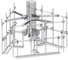
Monopole T-Frame kit with VSR Reinforcement and Work Platforms, 15 in to 50 in OD, 12 ft 6 in face, includes (12) 2-3/8in x 96in pipes
