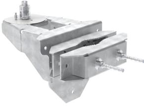
Mounting systems for cylindrical pipe installations (50-250mm pipe diameter) .Suitable for small cell cylindrical antennas with a weight less than 20KG and dimensions less than diameter\*height: 370\*610mm.
