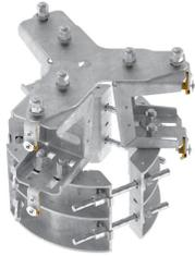
Pipe Mounting KIT with shroud, capability of mounting 37cm diameter round antennas (with trident mounting bracket, max length 2.1m, max weight 56kg) on the top of a pole with diameter from Ø150 to Ø273mm
