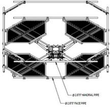
PIM Optimized Adjustable 4-Sector Monopole Platform with 13ft Face - 2-7/8in OD Face Pipes & Top Rail - No Antenna Pipes Included
