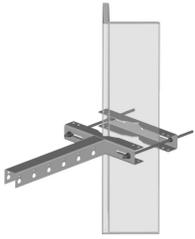
Star Support Tee Bracket for 1-1/2 in to 5-1/2 in OD round members and up to 5 in 90 degree and up to 7 in 60 degree angle members
